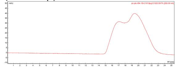
Analysis Method: Varian Prostar system with 1 ml/min DCM flow across one PLGel Mixed-D column and one PLGel Mixed-E column and one phenogel 5u column (Agilent). Detection via UV/Vis, calibrated against polystyrene standards.
